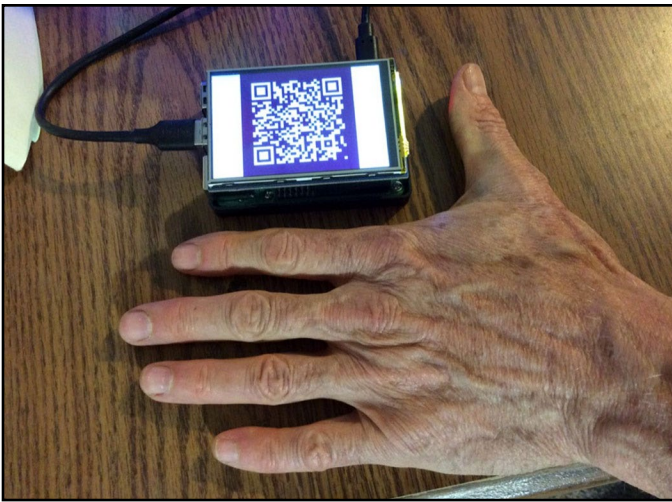
Figure 14. My RaspiBlitz: a combination of a $50 Raspberry Pi computer, free software, and $150 hard drive combine to create an online cash register and payment processing system.
